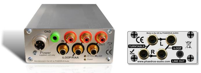
Connect the turntable to the **Groove Sleuth** preamplifier as described in the appropriate manual. Connect the **OUT** of the **Groove Sleuth Mk. II** or **Groove Sleuth LOCKDOWN** (LINE OUT for the **Groove Sleuth MICRO**) to the two inputs of the miniDSP **2X4HD**.
