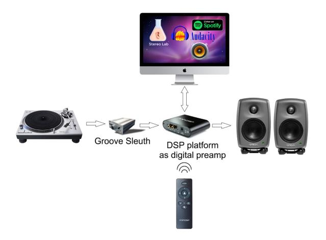
The third-party DSP platform may be used to implement RIAA equalisation (and other recording characteristics); as well as providing other preamplifier functions, such as source select and volume control (via IR remote).
